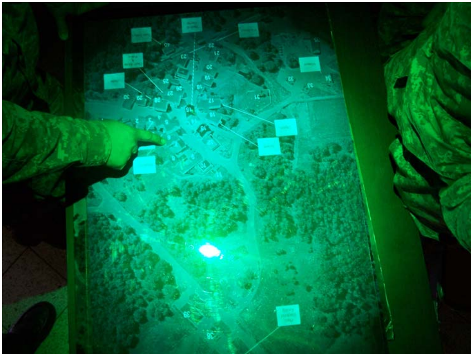
FIGURE 1.2 Army Research Laboratory’s tactical digital hologram technology, which is being used by special forces in Iraq and Afghanistan. The unit has a three-dimensional holographic display that incorporates human intelligence, terrain, and imagery data. SOURCE: U.S. Army Research Laboratory
