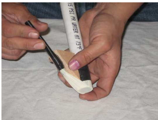
Figure 6-7. The wooden triangle secures the straw
