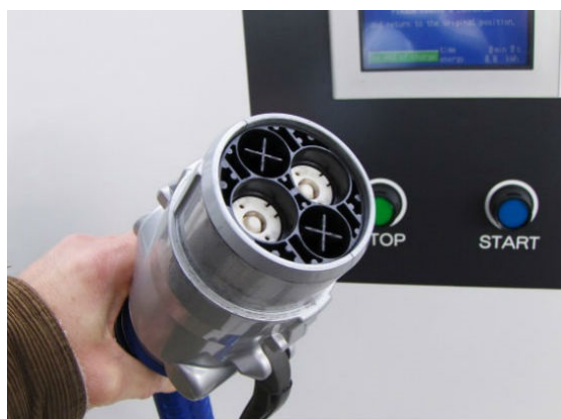
FIGURE D-2 The CHAdeMO plug for DC fast charging is used for most DC fast chargers now available in the United States, Europe, and Japan and is available on most BEVs that can accept DC fast charging. SOURCE: Brissette, 2013.
